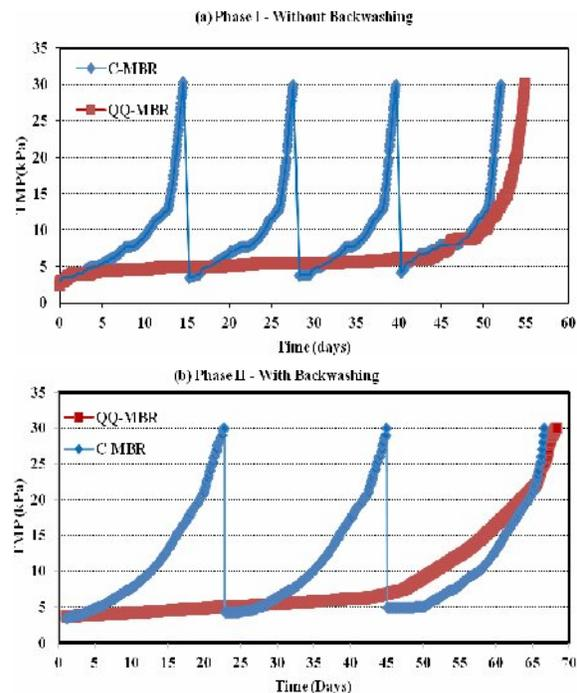
Fig. 2: TMP profiles of C-MBR and QQ-MBR; (a) Without Backwashing; (b) With Backwashing.
