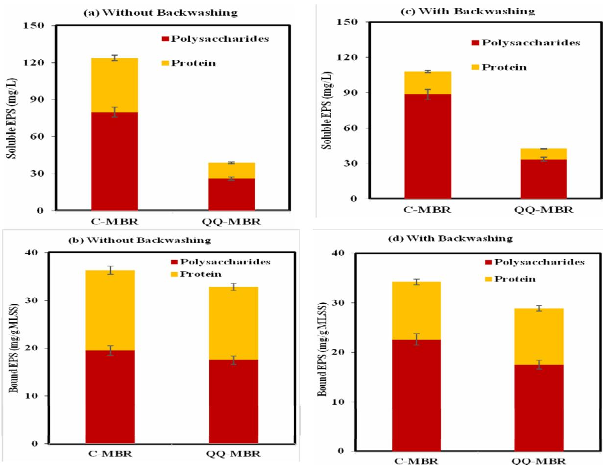
Fig. 3: (a) Soluble EPS in C-MBR and QQ-MBR without backwashing; (b) Bound EPS in C-MBR and QQ-MBR without backwashing; (c) Soluble EPS in C-MBR and QQ-MBR with backwashing; (d) Bound EPS in C-MBR and QQ-MBR with backwashing.
